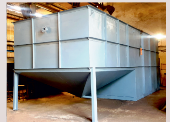
50KL STP Plant
